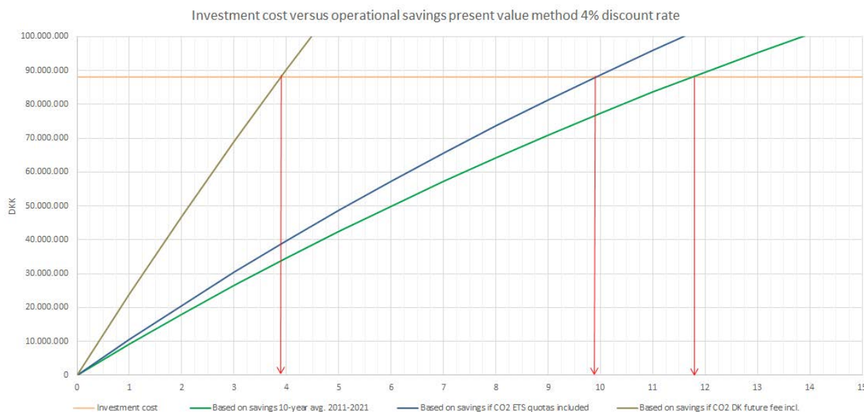
Figure 4.2.3 Accumulated savings discounted to present value with discount rate of 4% versus present investment cost incl. deductible VAT of 16% for shore-based charging stations. Source EMK.
