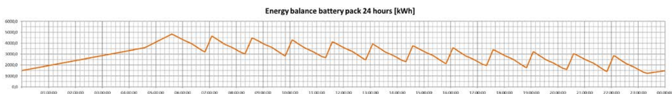
Figure 4.1.1 Energy balance or battery capacity used during a full day and night of operation with 12 single trips or 6 roundtrips for one E-Ferry Twin. Compiled by EMK.
